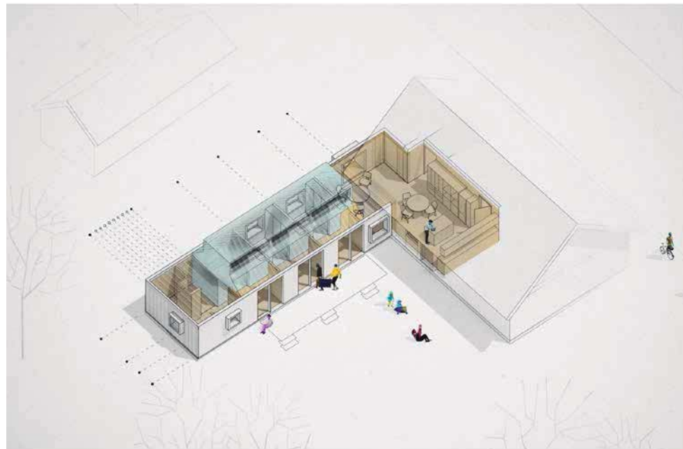
Transversal cut. The rooms are lit by the ceiling and a front window. to gain space, a bed lays over the corridor, making room for two people in a single room.
